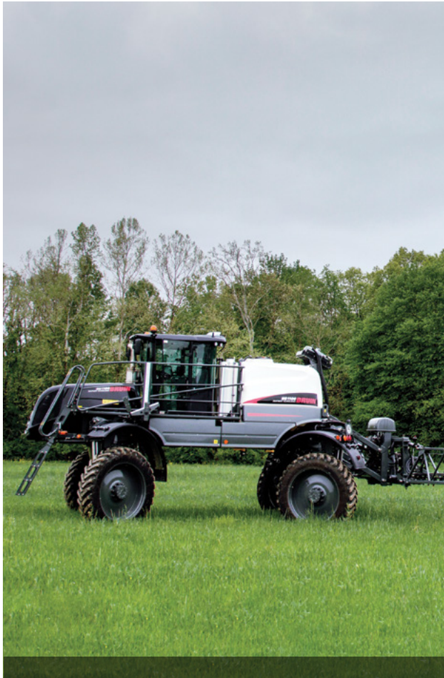
■ Four-Wheel Steer Four-wheel steering ensures that the rear wheels stay on the path and includes slope compensation with back axle correction for better control on hills and headlands. Crab steer mode allows for enhanced mobility in tight places.
