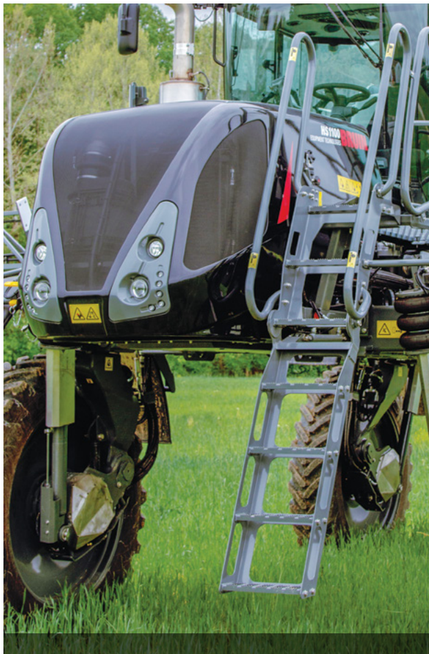
■ Front Ladder The front entry access ladder drops to just 16 inches off the ground making access easy. Disengaging the parking brake lifts the ladder into a field-ready position.
