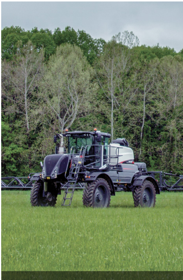
■ Hydrostatic Drive System The powerful hydrostatic drive system within Bruin Sprayers allow operators to choose between three drive modes: conventional hydrostatic control, eco-mode for better fuel efficiency, or standard foot pedal drive which is especially useful on the road.
