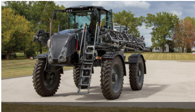
■ Narrow Transport A narrow axle configuration (79-105 inches manual, 90-120 inches hydraulic adjustment or 80 inches fixed) on the HS700 allows for easy transport between fields.
